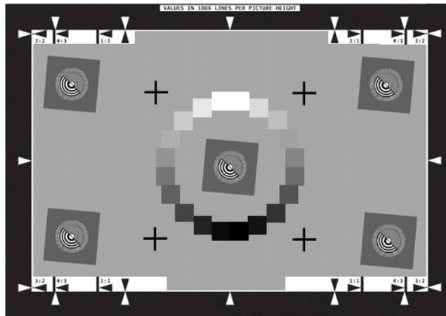
Figure 3: Proposed test target design for revised ISO 12233 standard with duplicate slanted-edge features
