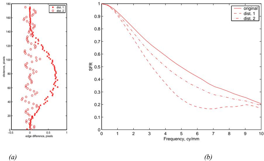
Figure 4: Example of the influence of optical distortion of camera edge-SFR measurements, from ref. 4. (a) Edge displacement observed because of barrel lens (1) and (2) ripple type distortion. (b) Measured SFR for undistorted edge. Sampling is at 400 ppi.
