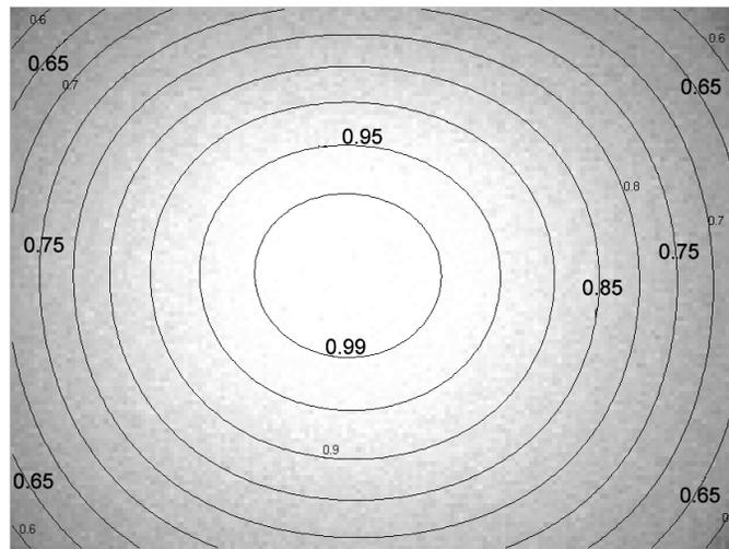
Figure 1: Example of cell phone camera (green-record) image due to a uniform field. The contour labels show the fractional level in the saved file, where the reference value was 246.3 (8-bit encoding).
