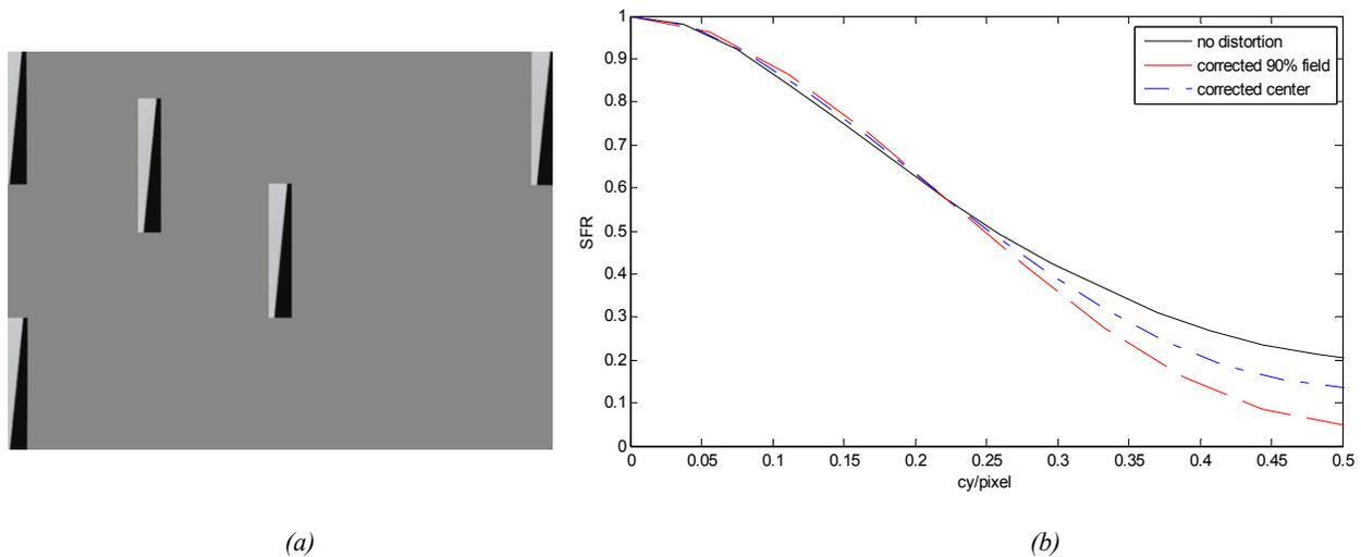
Figure 5: SFR results for a digital image before and after the barrel distortion correction (a) test image, (b) SFR results
