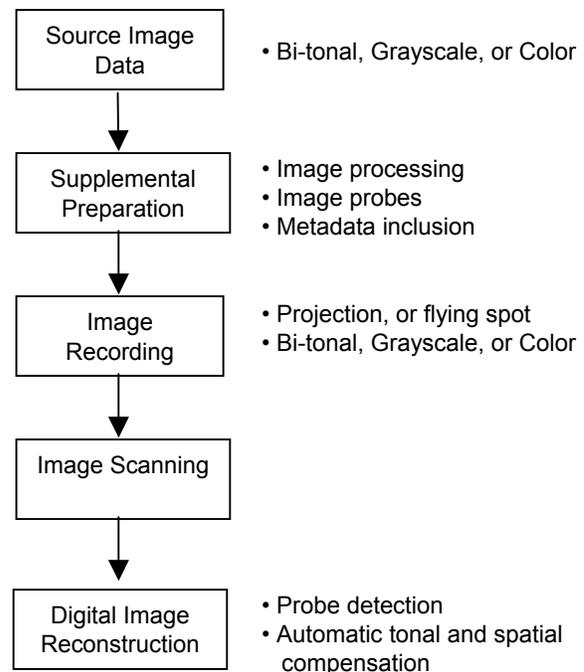
Figure 1: Imaging path for digital image archiving and retrieval with microfilm
