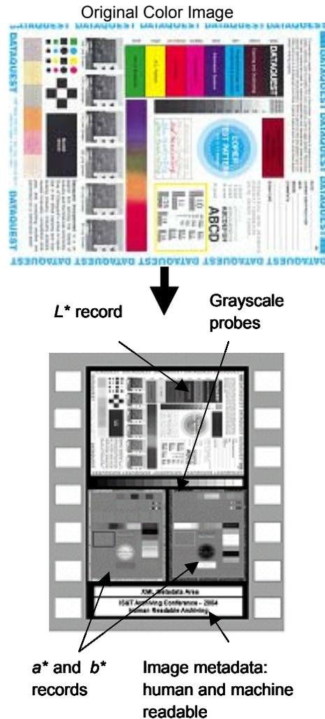
Figure 2: Color separation concept onto 35mm microfilm
