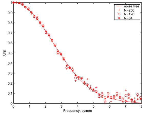
Figure 2: SFR measurements from simulated edge with image noise for varying data lengths
