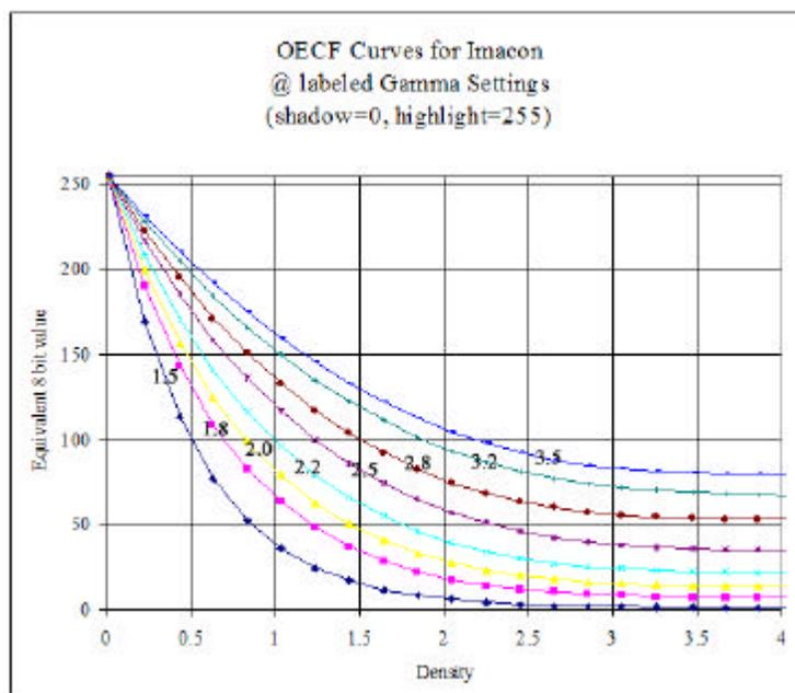
Figure 1 – Imacon OECF curves ; gamma 1.5 thru 3.5 ; color channel equivalence
