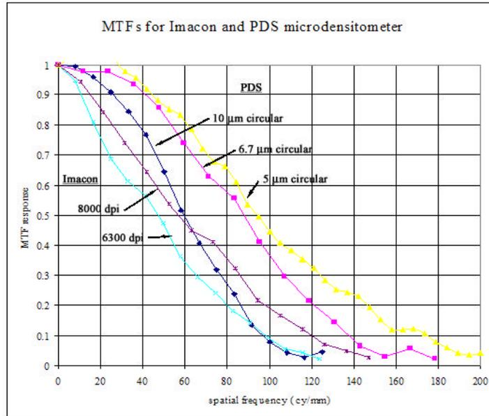
Figure 6 – MTF comparisons between Imacon and PDS microdensitometer
