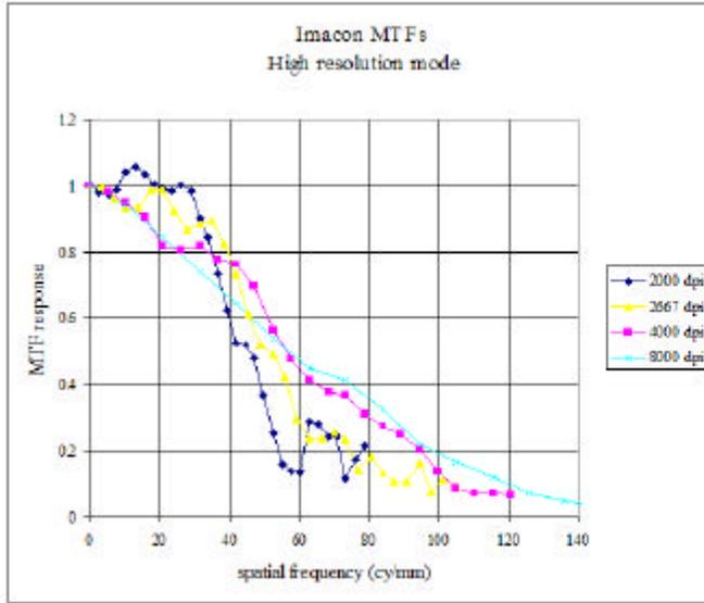
Figure 4 - High Resolution Imacon MTFs
