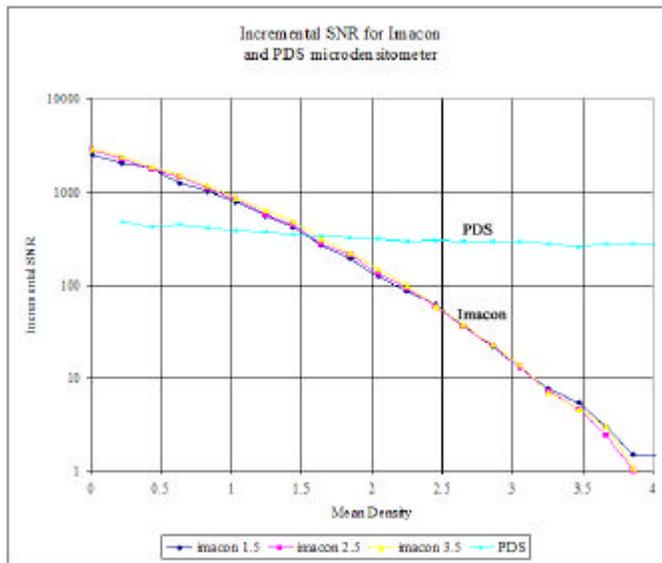
Figure 3 – Incremental\* SNR for Imacon and PDS microdensitometer
