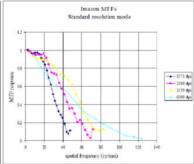
Figure 5 - Standard Resolution Imacon MTFs
