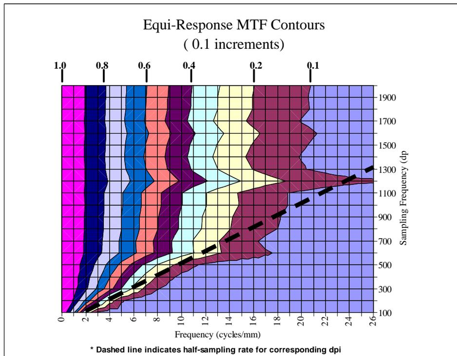
Figure 8 - MTF contour plots for flatbed scanner
