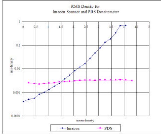
Figure 2 – RMS density for Imacon and PDS microdensitometer
