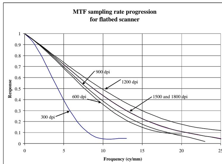
Figure 7 – MTF sampling rate progression for candidate flatbed scanner
